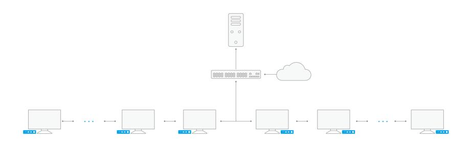
vCloudPoint zero client computing solutions are innovative desktop computing solutions that shift the traditional PC computing infrastructure to a centralized computing model. Within a zero client computing solution, users replaces PC desktops or laptops with the access client devices, called zero clients, to remotely connect to virtual desktops centrally hosted in the servers at the data center.
